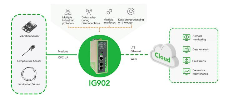
InHand Networks offers a remote monitoring solution for bearings featuring its InGateway902 industrial edge computing gateway, helping collect data of the bearing status (vibration, lubrication, temperature, abrasion, etc.) and upload them to the cloud for analysis and preventive maintenance.
